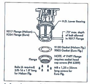
Securely connect SR200 Big Gun to traveller or riser designed to handle the loads of the operating sprinkler. Take care not to bottom out the bolts in the flange yet allow for at least 1/2" engagement of the bolt threads.
