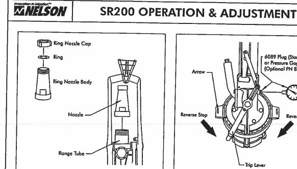
2. Install Nozzle on end of Range Tube. If using a Ring Nozzle, Install desired Ring size in Cap. Assure Ring is centered. Ring Nozzle Cap and Nozzle can be sufficiently tightened by hand.
