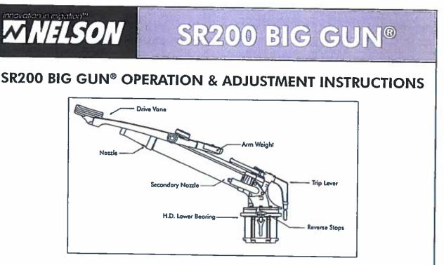
NOTE ON LUBRICATION: The SR200 sprinkler is lifetime lubricated and does not require periodic lubrication. The ball bearings in the H.D. lower bearing operate in a water resistant lubricant that is packed in the housing cavities and retained by seals. If repair of the lower bearing is done, it is recommended to use Nelson #6143 lubricant or a good grade of water resistant lubricant such as Lubriplate 130-AA.
