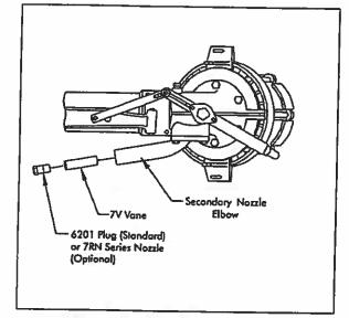
5. The SR200 is capable of using a Secondary Nozzle for in-close coverage. To use this feature, remove the supplied 6201 Plug and replace with the 7RN Series Nozzle of your choice. The supplied 7V Vane must be used to maintain proper stream integrity.
