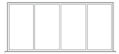
2. Inappropriate Replacement Window Proportions
