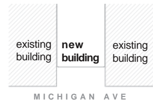
Plan: “Facade Set Back from Streetwall” Not-Appropriate: New Building Disengaged from Streetwall
