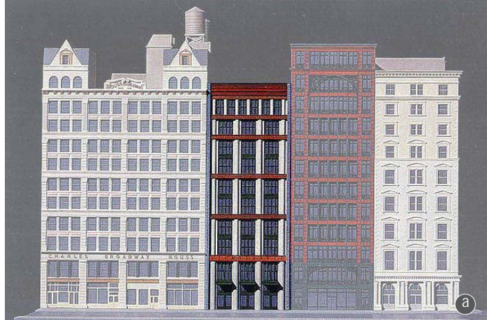
This infill building (center) is exemplary in its understanding of design elements such as scale, height and massing, materials and facade design within the context of its surroundings. Retail storefronts articulate the base to blend with the retail nature of its context. The middle expression is one of masonry piers subdivided by windows with characteristics similar to the scale of the neighborhood. The cornice is further accentuated in terms of scale and materials.
