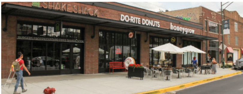
Example of new commercial development on intersecting streets with an industrial building context. The facade incorporates flat metal awnings and floor to ceiling window displays, punched through the brick with hanging placard signage (Lake and Morgan).
