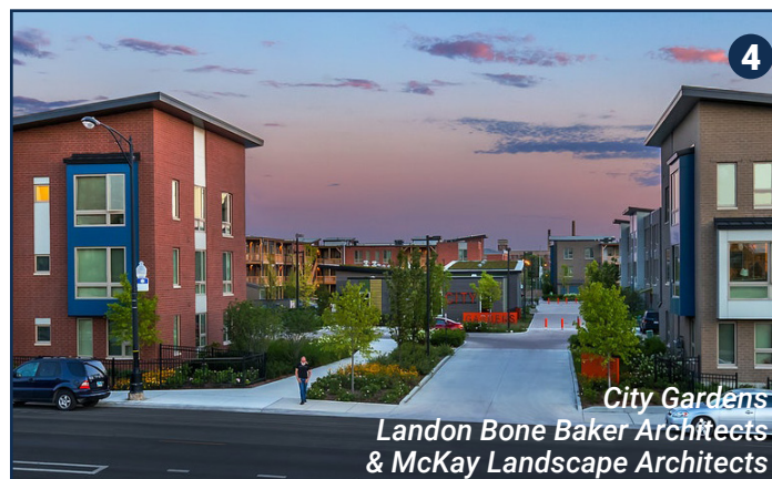
Separating pedestrian and vehicular entrances with quality planting helps demarcate space and avoid conflicts.
