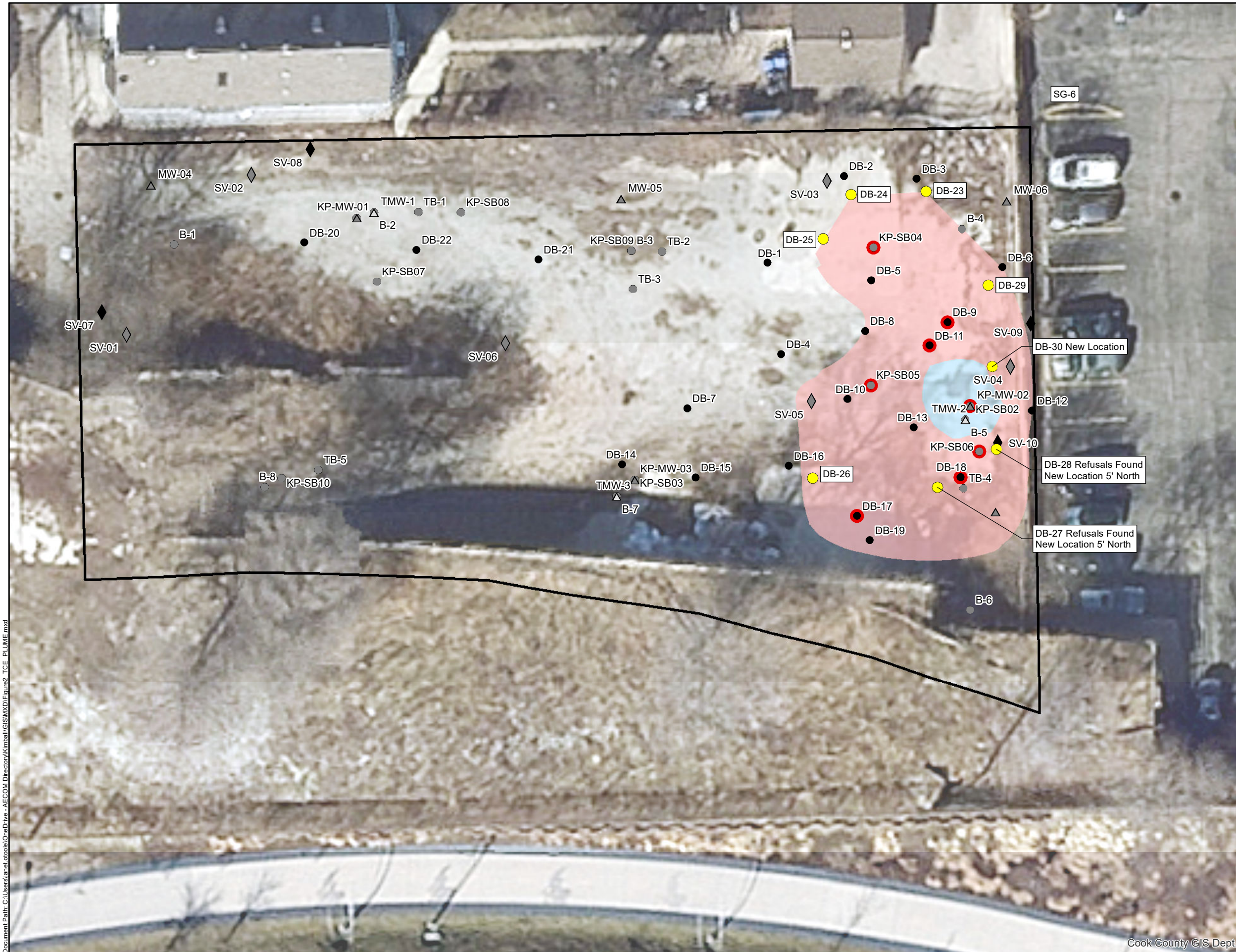
FIGURE 2-2 SAMPLE LOCATION AND SOIL EXCEEDING TCE C_{SAT} LIMIT MAP
