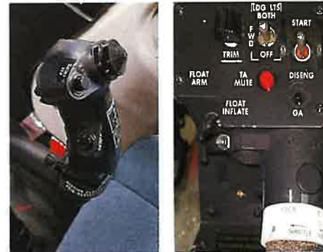
Figure 2-7. Cyclic and Collective Stick. Both crew stations have access to basic cyclic and collective flight controls.
