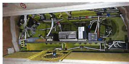
Figure 2-2. Expanded Avionics Shelf. The Expanded Avionics Shelf for the installation of additional avionics and other mission-related equipment.
