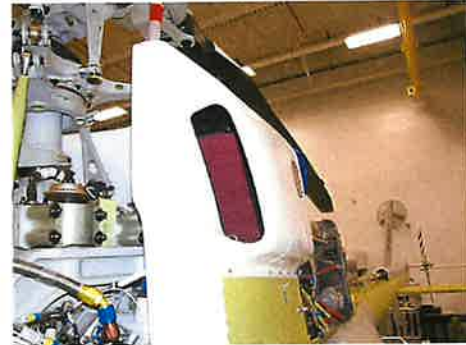
Figure 2-21. Inlet Barrier Filter with Access Door.
