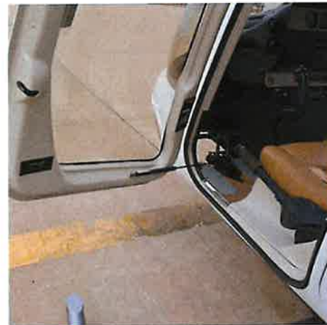
Figure 2-16. Automatic Door Openers for Hi-Viz Crew Doors.
