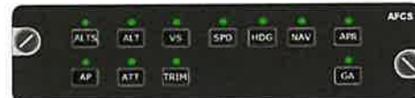
Figure 2-10. AFCS Control Panel in Center Console. The crew selects the modes needed for flight by using the AFCS control panel.
