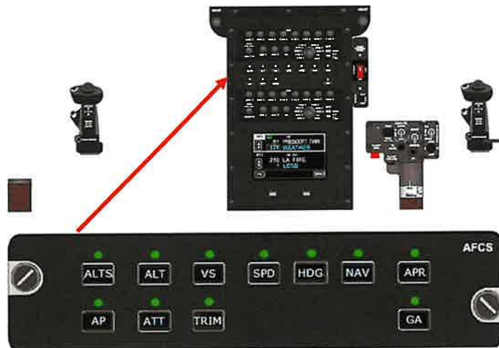
Figure 2-6. Autopilot Control Panel and Grip Controls. The AFCS controls are accessible to both pilots.
