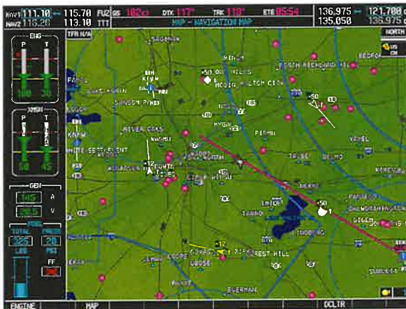
Multi-function Display (MFD) displays engine, communication, navigation, traffic, weather
