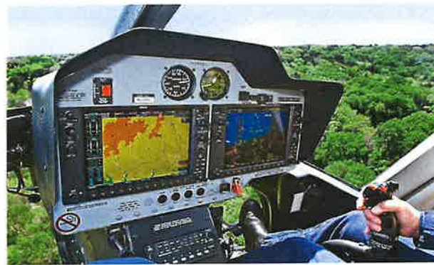
Figure 1-5. Integrated Avionics Suite. The Garmin Integrated Avionics Suite reduces pilot workload through the incorporation of all functionalities in two 10.4" displays, resulting in increased crew and passenger safety.
