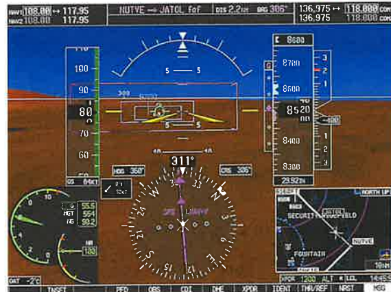
The Primary Flight Display (PFD) graphically summarizes all critical flight information
