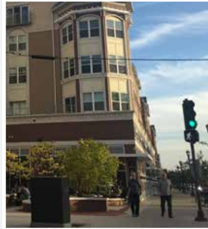
A building setback above the building base frames the street and establishes a comfortable pedestrian experience
