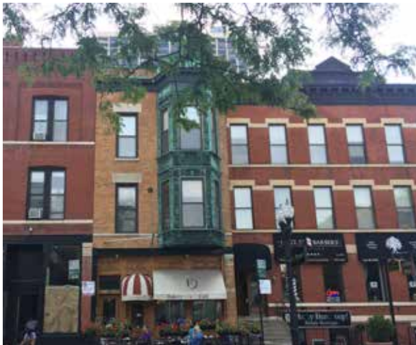
Promote variety through changing the use of materials, roof lines, and windows to create a sense of rhythm.
