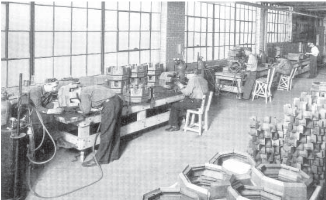
In the 1930s, White Castle switched from white-glazed brick to standardized white porcelain-enamel steel panels for building exteriors. Top: A porcelain-enamel steel-clad White Castle on Hempstead Turnpike in New York City's borough of Queens, photo from 1936. Bottom: A view of workers building castellated details for White Castles in the Porcelain Steel Buildings factory in Columbus, Ohio (date of photo unknown). In order to control costs and ensure quality, Ingram established Porcelain Steel Buildings as a wholly-owned subsidiary to manufacture the porcelain-enamel steel panels used in these later White Castles.
