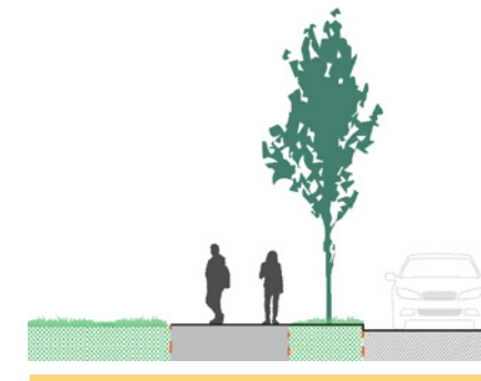
Figure 42. Residential ROW with trees in sodded parkway planters
