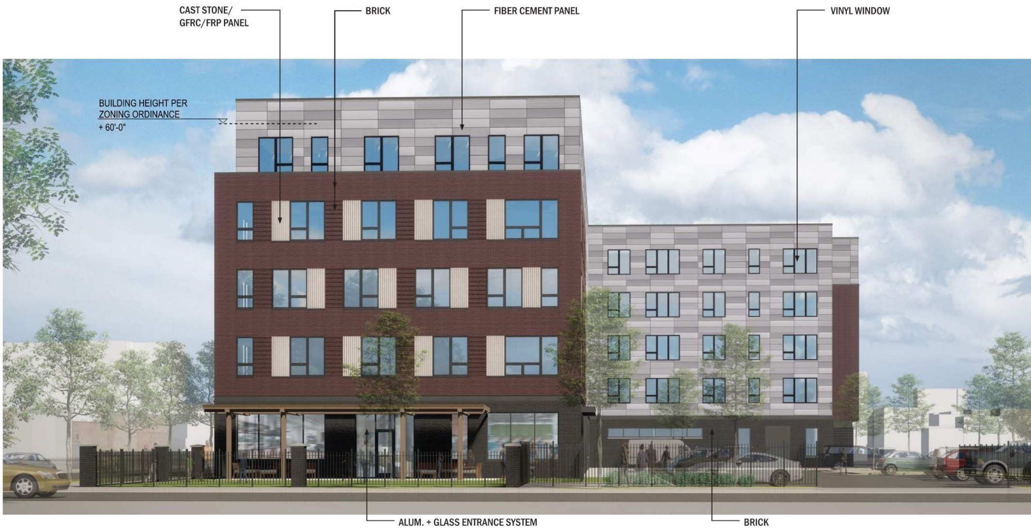
BUILDING ELEVATION (SOUTH)
