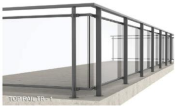
Second Level Railings and Posts with glass infill panels. Railing systems sits behind Second level parapet.
