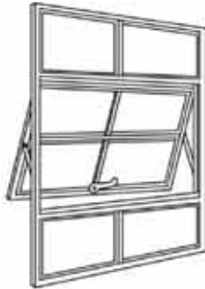
STEEL WINDOW WITH OPERABLE SASH
