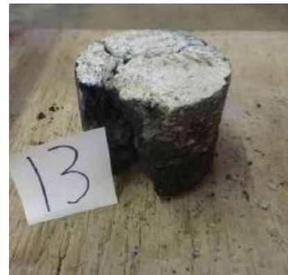
Asphalt Pavement Core (from Drilling Rig)
