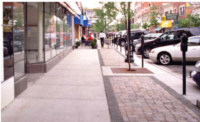
Figure 4-39: Standard sidewalk with unit paver border
