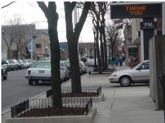
Figure 4-30: Standard railing on planter curb
