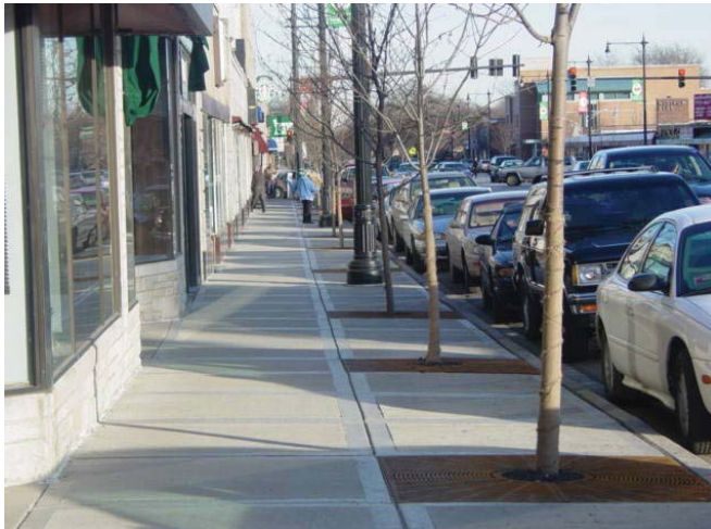
Figure 2-15: The repetition of trees in grates and streetlights along the block creates the “module”
