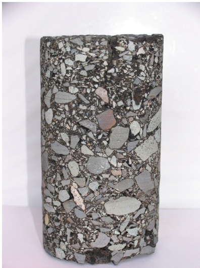
Test Section Pavement Core
