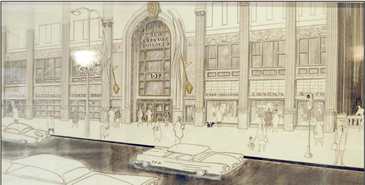
The Old Republic Building has an imposing entrance for tenants and their guests. The entry doors are within a monumental three-story arch, with a surround featuring rope moldings and floral designs. At the top are swags and a cartouche with the initials of the building. Top: Photo of entry, ca. 1924, showing four-story base and three-story monumental arched opening. Bottom: Rendering of entry, ca. 1957, after the purchase of the building by the Old Republic Insurance Company.
