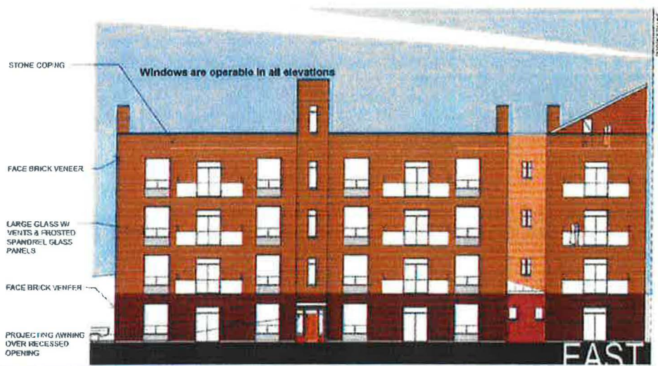
Figure 5-3: BUILDING ELEVATION - EAST
