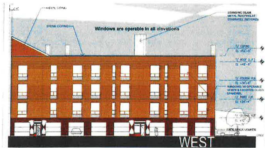
Figure 5-6: BUILDING ELEVATION - WEST
