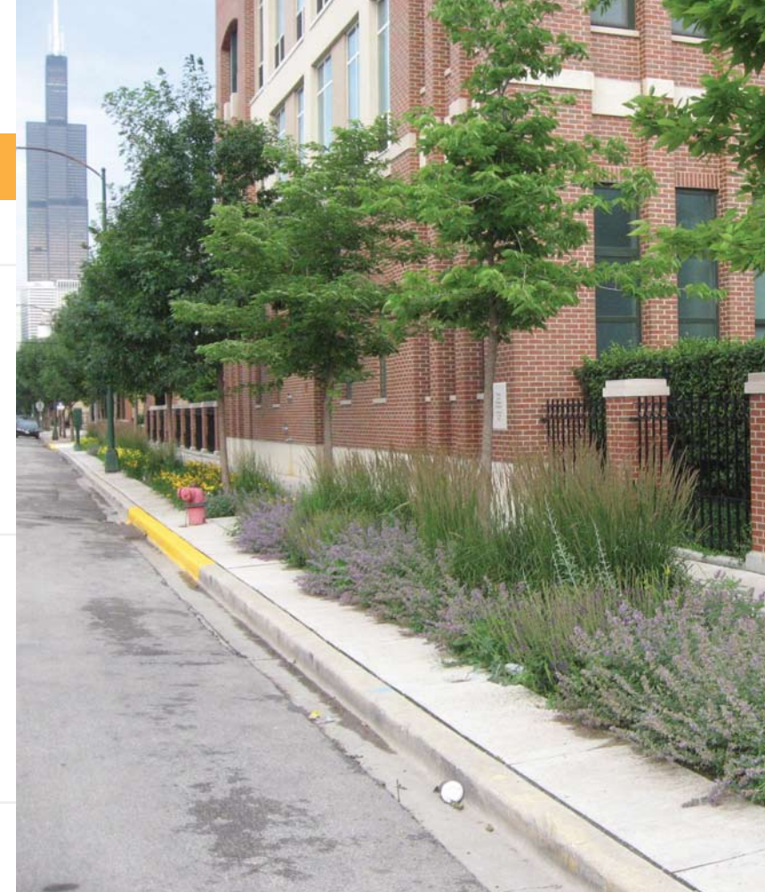
This landscaped parkway was designed to collect stormwater from the sidewalk, sending less to Chicago's combined sewer system.
