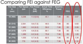
Includes drive losses; more accurate to system efficiency rather than component efficiency
