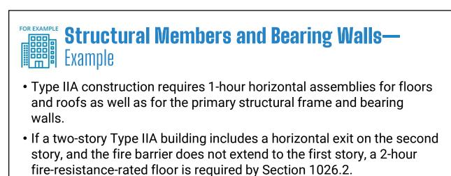
• The primary structural frame and/or bearing wall structure supporting this floor must also have a 2-hour fire-resistance rating per Section 704.1.
