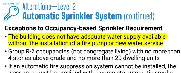
If an automatic fire suppression system cannot be installed, the work area must be provided with a complete automatic smoke detection system throughout all occupiable spaces except for sleeping units or individual dwelling units
