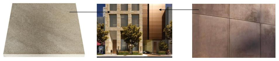
NATURAL LIMESTONE Proposed cladding on levels 01-06 METAL PANEL Proposed cladding on levels 01-06 and on balconies
