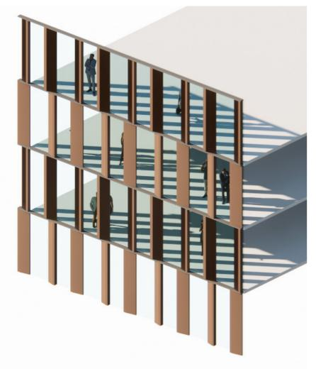
1. Folded metal panel facade alternating floor to floor
