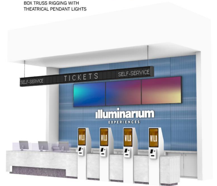
TICKETING COUNTER WITH CONCRETE FACE AND COUNTER TOP, BACK-LIT ROUTED RESIN, DIGITAL DISPLAYS, AND FACELIT BRAND SIGNAGE
