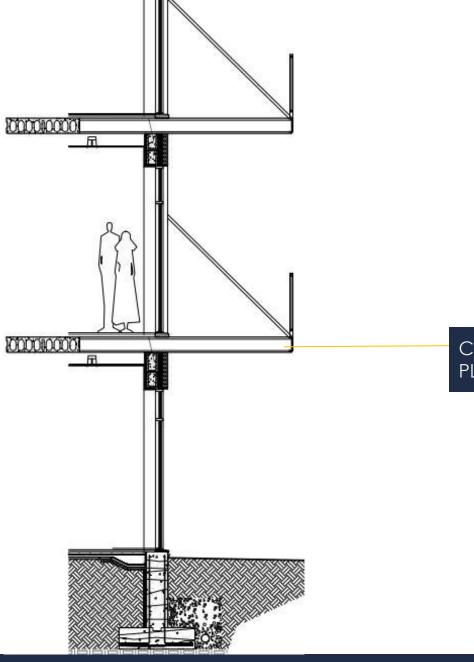
CANTILEVERED CONCRETE PLANK BALCONIES
