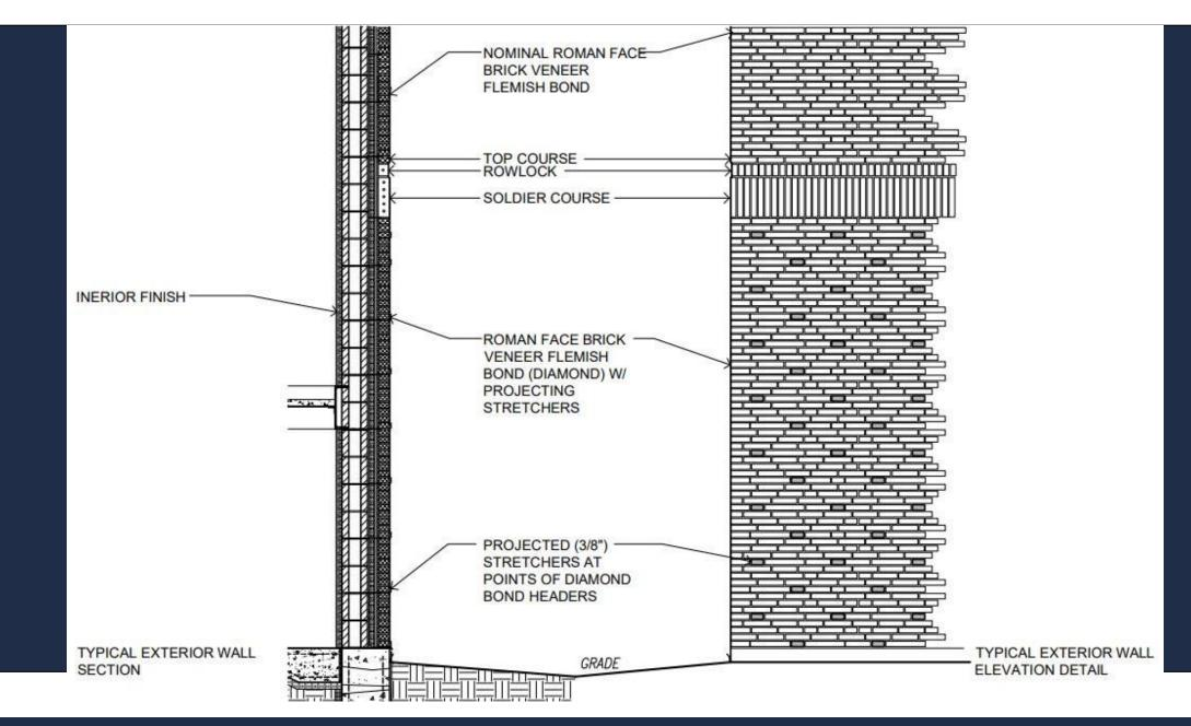
FAÇADE SECTION & FAÇADE DETAIL ELEVATION 37
