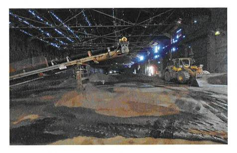
COMMENTS: September 1, 2021 - Foundry Sand operations. Accumulation of fine materials on floor and holes in the ceiling/roof.
