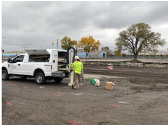
Photo 3: Boring advancement using a GeoProbe on the east portion of the site facing north.
