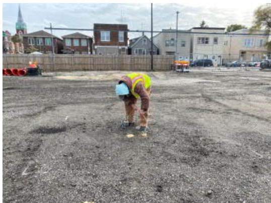
Photo 5: Soil gas sampling with a Suma canister facing south.
