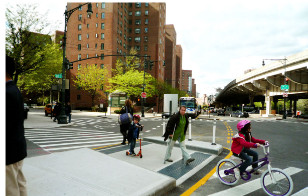
Pedestrian refuge island New York, NY Source: NYC Department of Transportation
