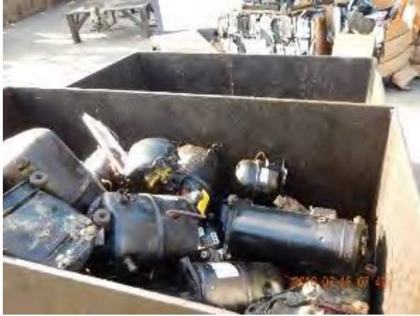
Compressors removed from refrigerators and other appliances, Ecology, Colton, CA.
