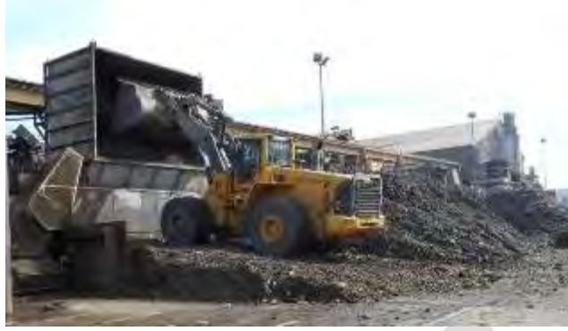
Front loader used to feed stockpiled aggregate into the joint products plant, Schnitzer Steel, Inc., Oakland, CA.
