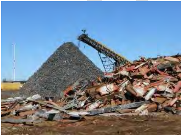
Pile of sorted ferrous metal, background, and scrap metal from the Oakland Bay Bridge demolition project, foreground, Schnitzer Steel, Inc., Oakland, CA.
