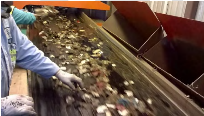
Hand picking station, Sims Metals, Redwood City, CA.
