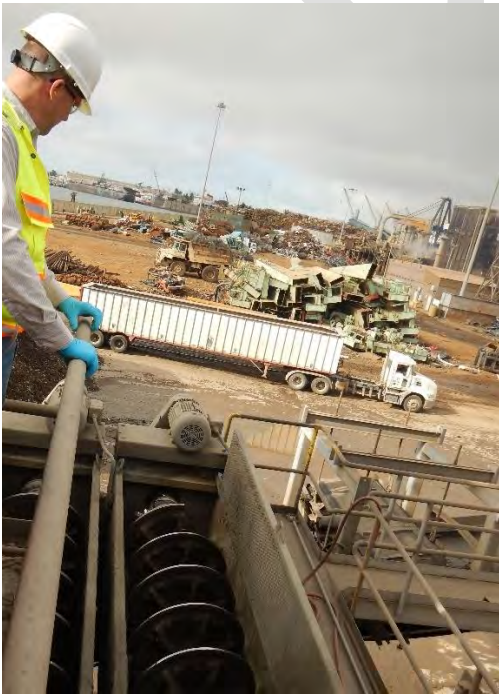
Pug mill mixing screw at Schnitzer Steel, Oakland.
