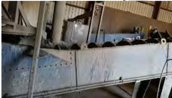
Pug mill mixing screw, chemical treatment of metal shredder residue, Sims Metal Management, Redwood City, CA
