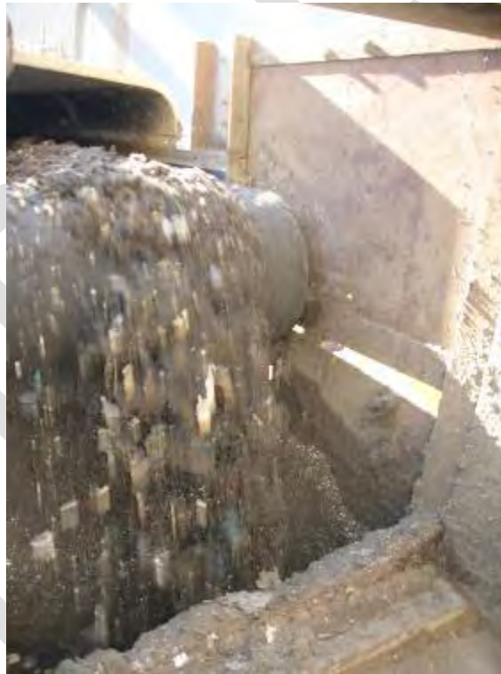
Metal shredder residue exiting the joint products plant following removal of non-ferrous metals
