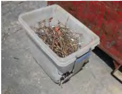
Waste mercury switches pulled from appliances, Ecology Auto Parts, Colton, CA.
