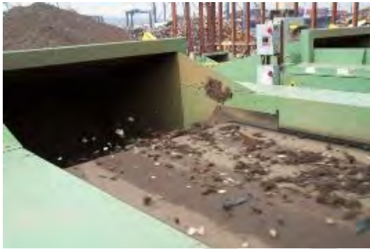
Eddy current separator, used for recovery of non-ferrous metals.
