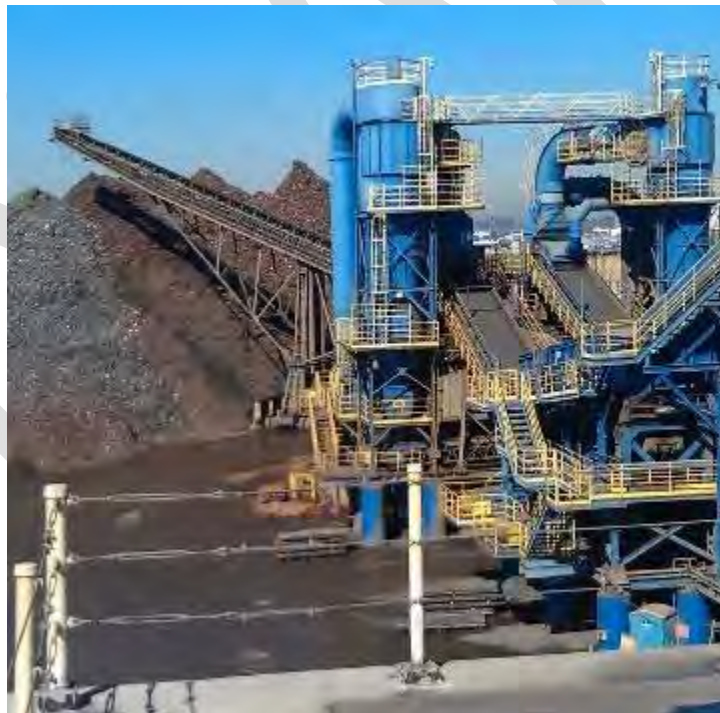
Pile of sorted ferrous metal following shredding of scrap metal at SA Terminal Island.
