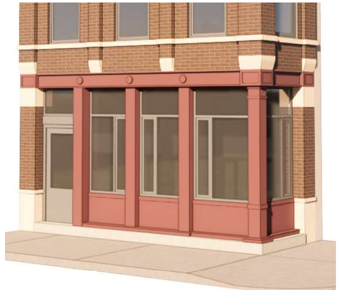
Replace corner entry by extending the storefront window system to the corner
