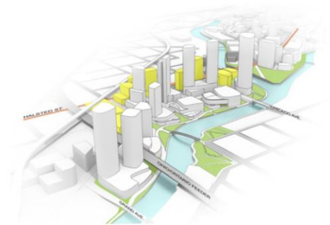
STEP DOWN HEIGHT OF BUILDINGS TO TRANSITION TO SCALE OF ADJACENT NEIGHBORHOODS
