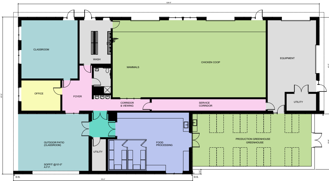
1 BARN / GREENHOUSE - FLOOR PLAN 3/16" = 1'-0"
