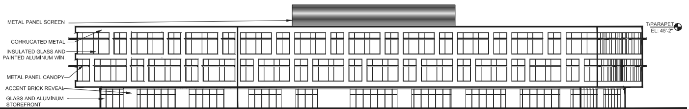
BUILDING B1 3 STORY OFFICE WITH GROUND FLOOR RETAIL SOUTH ELEVATION - FACING OGDEN
