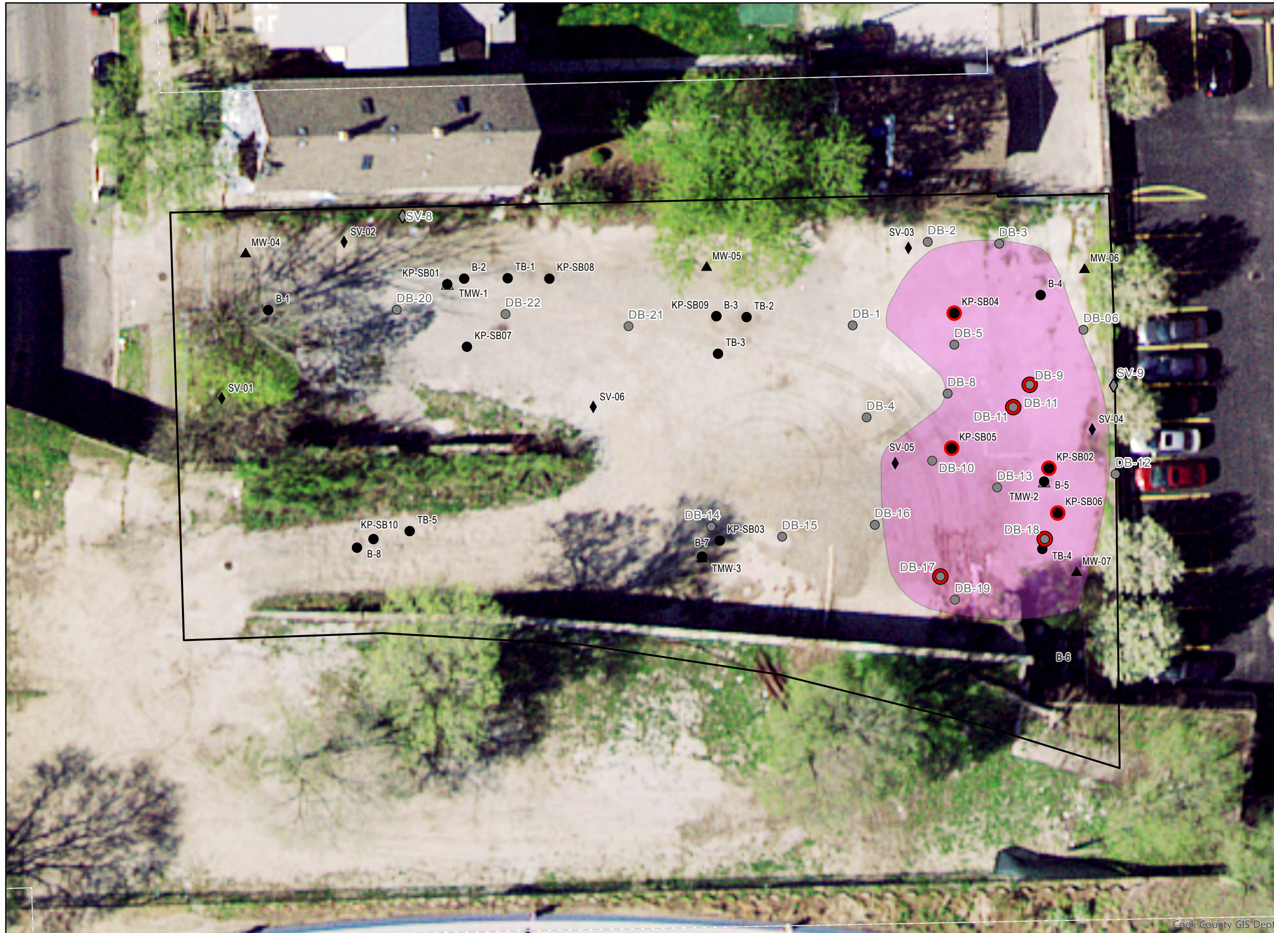
Figure 2-2 Sample Location and Soil Exceeding TCE C_{sat} Limit Map
